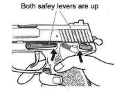
When hammer is not pulled back, single safey is available at the front lever
